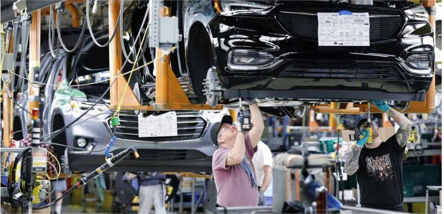
The automotive industry involves a lot of underbody shot work to tighten bolts or drive screws on the underside of vehicles. Performing these tasks manually, especially on an assembly line, means an employee is holding a tool at or above shoulder level repeatedly over long periods of time. The employee must also deal with tool torque and contorting to work on hard-to-reach places when doing underbody shots.
